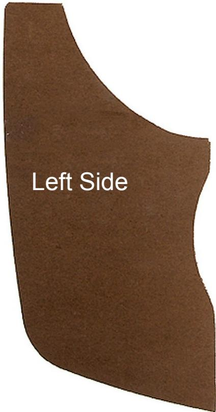
These are the next panels to go into the trunk. Put the left side in by matching the cutout with the hump near the bottom of the wheel well tub. Be careful not to break the panel by forcing the piece into place. Start by sliding the front of the panel under the edge of the trunk fender then slide the cutout into place. The panels should fit under the edge of the trunk lip. The side panels should be on top of the floor panel on both sides.
