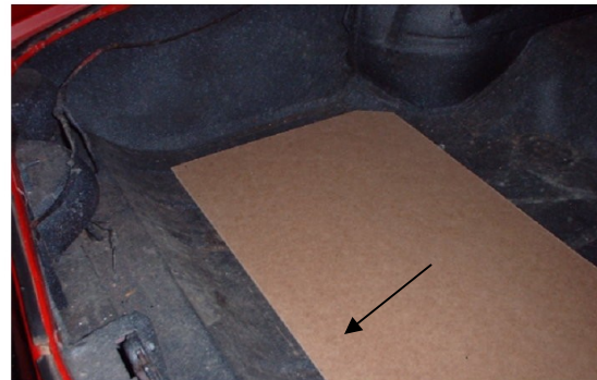
On the left side move the panel back against the upslope of the trunk, note the arrow.
