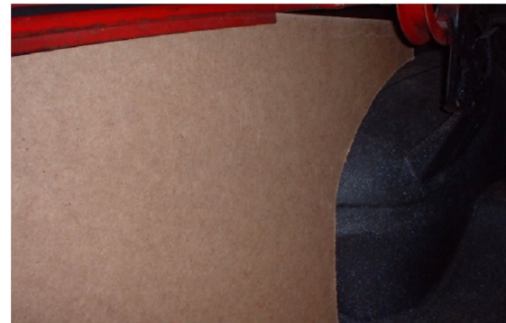
On the left side move the panel back against the light housing for a better fit.
