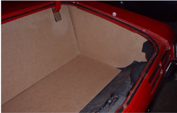
You now have 4 panels in place and will need to finish the trunk off with the back trunk latch panel.
