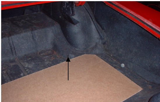
The first panel in fits right up to the jack hold down on the right side of the trunk. Note the arrow with panel in front of the hold down bracket.
