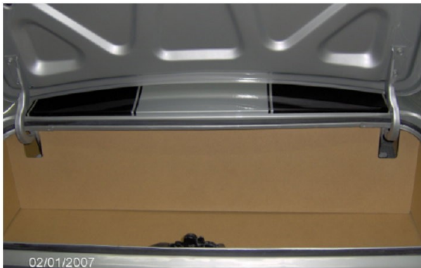
The final piece is the rear panel. Carefully put the panel in tilted to the rear, bottom first and then move it up into place.
