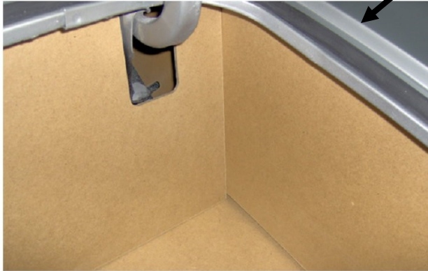
The right panel is in place. Pull the side panel up against the lip of the trunk for a good fit. The arrow indicates the lip where it should fit
