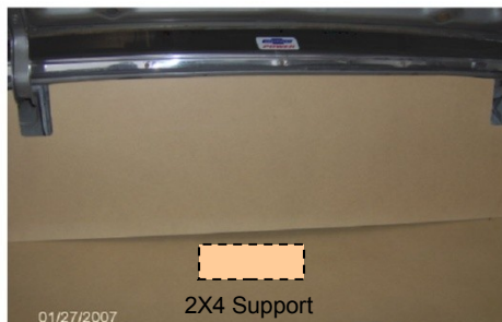
Note the dip in the center of floor panel. You will need to add support by using 2X4's or one 4X4.
