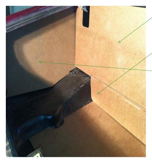
panel making sure to slide it in at the top first and then slide the bottom of the panel so the there is a slight lean to the rear of the trunk, note the picture. Next install the covered two side panels on the left and right side of the trunk. The side panels will need to be up against the lip of the trunk and pushed back against the lights.
