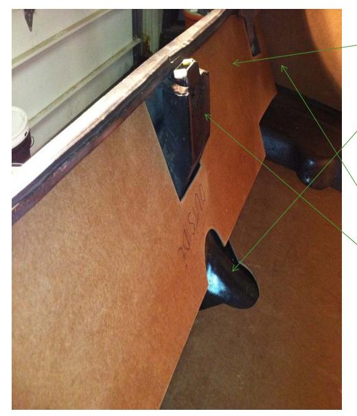
The last covered panel to go in is the trunk latch panel. Note that the panel only fits one way before covering this panel. The small area exposing the gas filler neck will also need to be covered. Note that the latch panel fits up under the lip of the trunk. The side panels fit against the latch panel, see the picture. You may want to paint the exposed latch and the braces on the right and left side of the trunk first before installing any panels.
