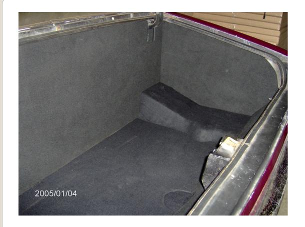
This is the finished right side of the trunk. Note that the gas filler area is covered and the floor fits on top of it.
