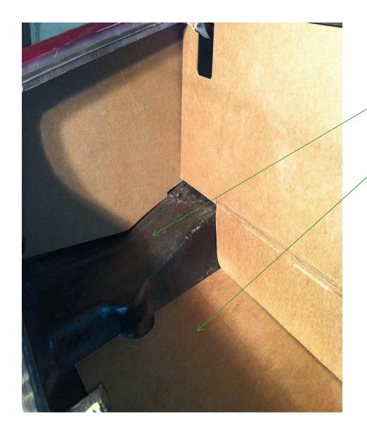
Test fit all of the panels to insure that they will fit correctly. The first thing to do is cover the spaces that are metal with material. The right and left side will need material applied. Measure past the latch panel and under the floor panel. Once that is complete, cover the floor with your material of choice, carpet or the material selected for all of the other panels. The floor is the first panel installed once the metal sides are covered.
