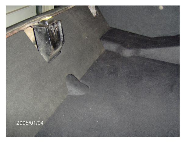
This picture shows the finished back latch panel. The side panels fit on the edge of the back latch panel. The back panel also fits under the rear lip of the trunk and against the edge of the floor panel.
