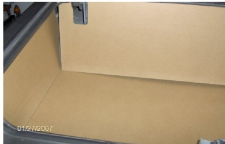
4. Rear trunk panel installed last.
