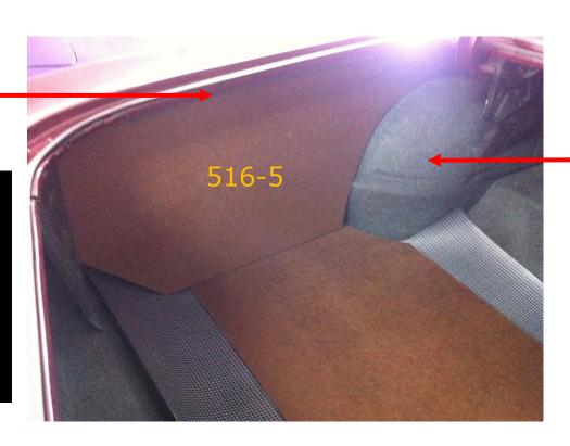
The next panel in is the hinge panel. It goes in top first with the bottom tilted back and then slide the panel in from the bottom. This panel will be on top of the floor panel and under the edge of the trunk.
