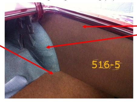
The next piece to go is the left side panel. It's the same as the right, it will sit on top of the floor panel. This will get tricky because there is nothing to hold them in place. They will rest under and against the lip of the trunk. See the picture for detail.
