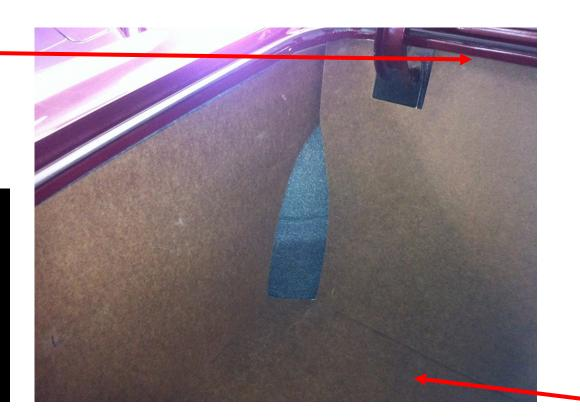
The last panel installed is the trunk latch panel. The two thin edges of this panel are the easiest pieces that can break, handle this panel carefully. Slide the panel in under the lip of the trunk. The panel will set outside of the right and left fender panel and should be flush against the latch panel. The final step is to rest on the back edge of the floor panel against the floor panel. See the pictures for fitment.
